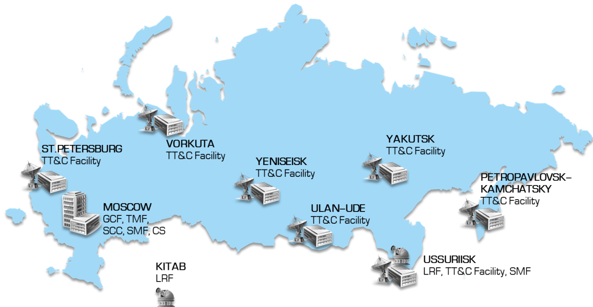
Figure 1.5.2 — The GLONASS Command and Control Subsystem
